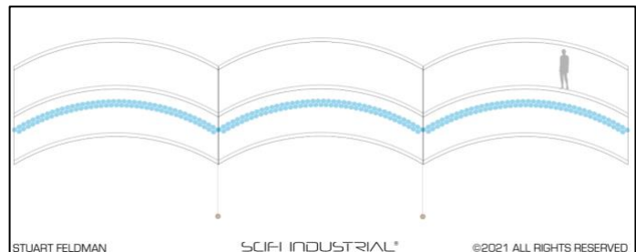
Figure 4. The canopy over Parks, N-S cross-section comprises three layers of 3 mil PET, with reinforced fibers. (Feldman)
