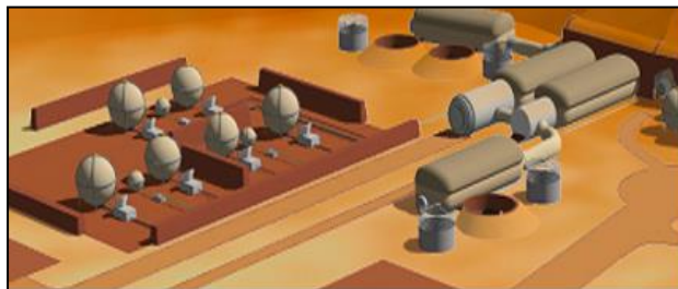
Figure 17. Fuel Production at Launch Site, nuclear reactors, storage for CO fuel and LOX, and repair shops (G. Petrov)
