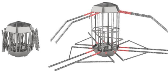
Figure 4. Extending girders in compacted and deployed state. The extended parts are marked in red. More on the necessity of these parts can be found in section E.
