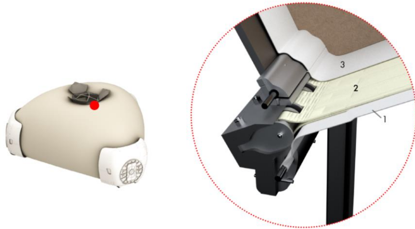
Figure 6. Model overview from the outside with detail position marked in red (left). Connection detail of the membrane with the upper core structure (right). This is an abstracted example showcasing a possible construction approach. The other connection points can be adaptations of the one showcased above. 1. interior layer with air bladders separated by Kevlar felt layers and interior finish; 2. restraint layer made up of Kevlar belts; 3. outer layer made up of chambers filled with regolith.
