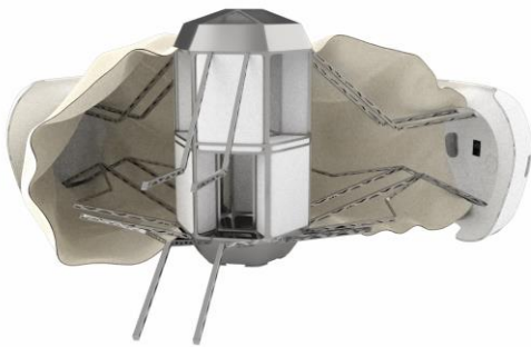
Figure 11. Section of habitat during deployment process
