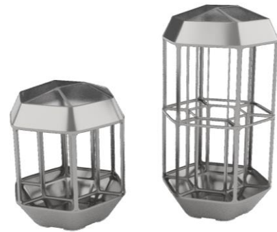
Figure 3. Telescopic core in compacted and deployed state
