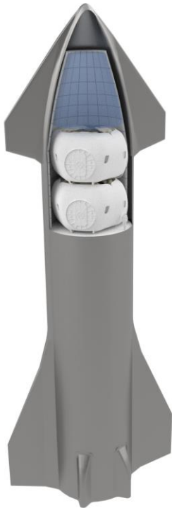
Figure 8. Starship cargo space with two stacked habitats in compacted state. The remaining space (marked in blue) can be used to transport the remaining necessary fixtures.
