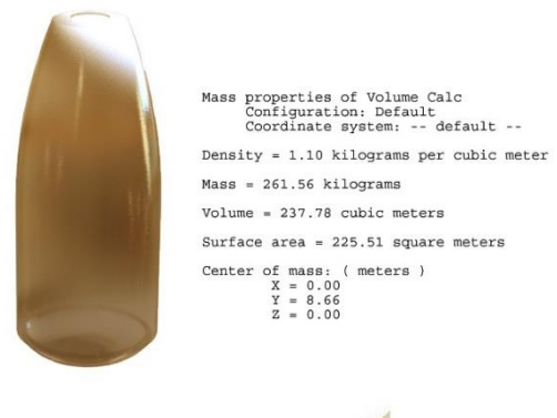
Figure 7. SW Air calculation of Ariane 5 PFSS
