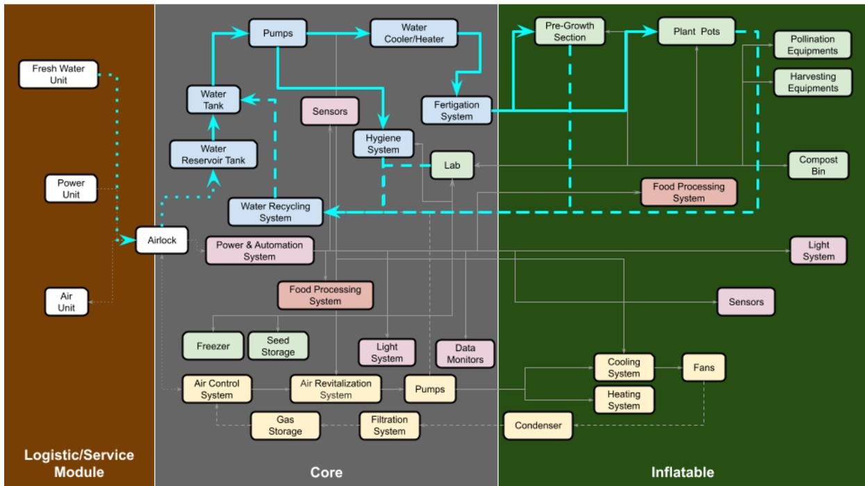
**Figure 4 Greenhouse Systems Water Circulation Diagram (the continuous lines are clean water, dashed are gray and black water, and the dotted lines are water supply from LSM module)**
