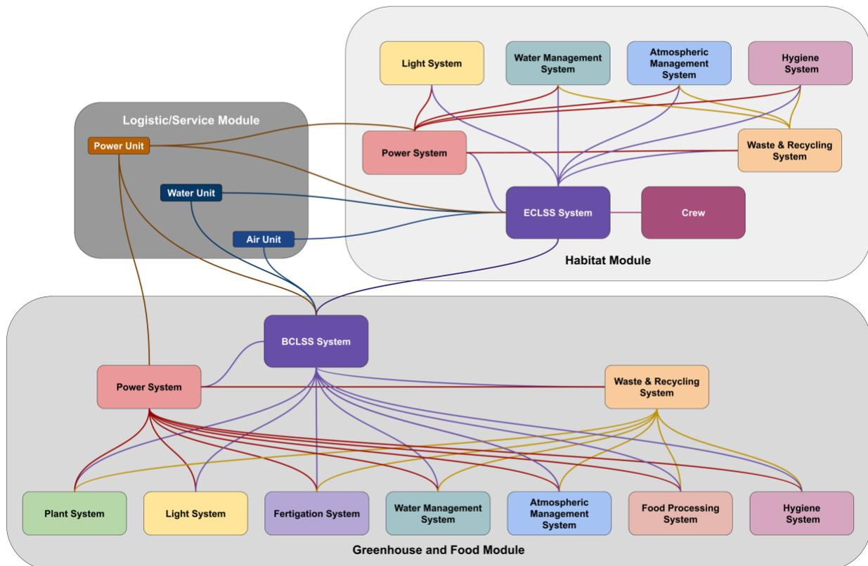
**Figure 1 Systems Integration Diagram**
