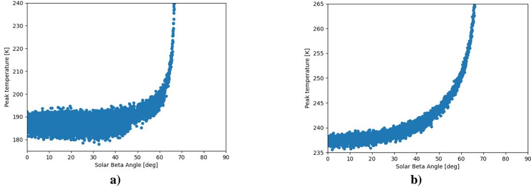
**Figure 6. a) Minimum peak temperatures for the a) lowest (310 s) and b) highest (2480 s) characteristic time as a function of the SBA.**
