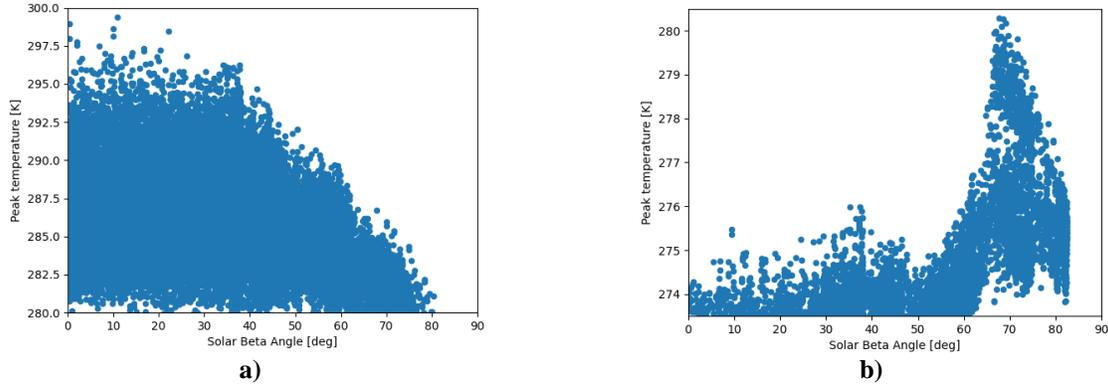
**Figure 5. a) Maximum peak temperatures for the a) lowest (310 s) and b) highest (2480 s) characteristic time as a function of the SBA.**
