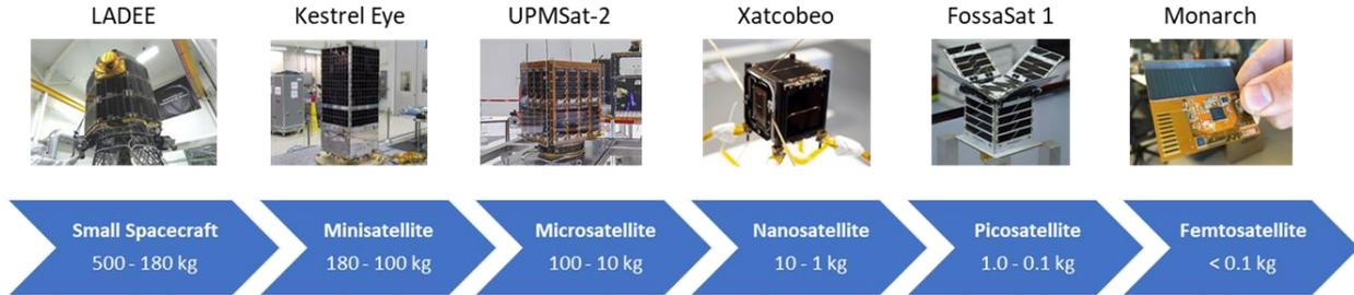
**Figure 3. Miniaturization process in the space system designs.**
