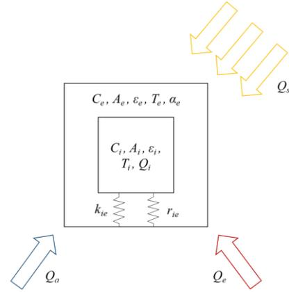
**Figure 9. Scheme of the thermal model used in ESATAN-TMS.**
