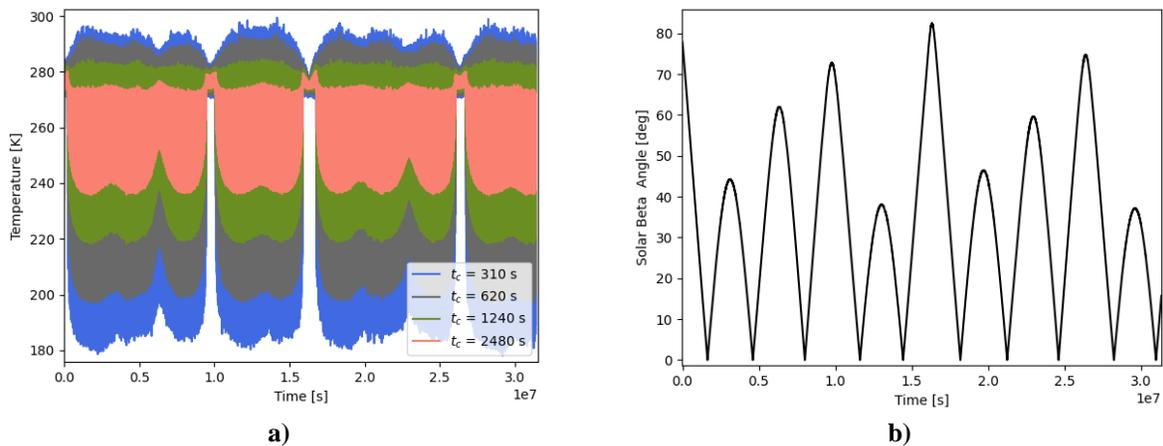
**Figure 4. a) Temperature and b) SBA evolution for the considered orbit during a whole year.**
