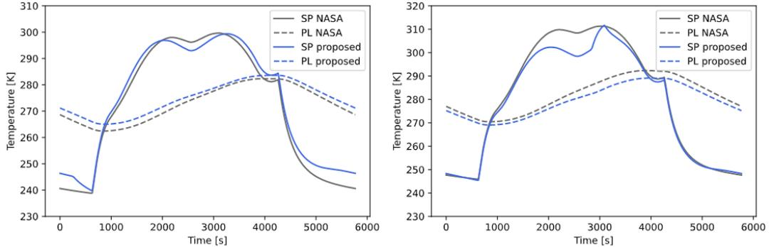
**Figure 10. Case 1 (decoupled nodes) thermal model temperature response for the coldest (left) and hottest (right) worst-cases using NASA and time-dependent proposed criteria.**
