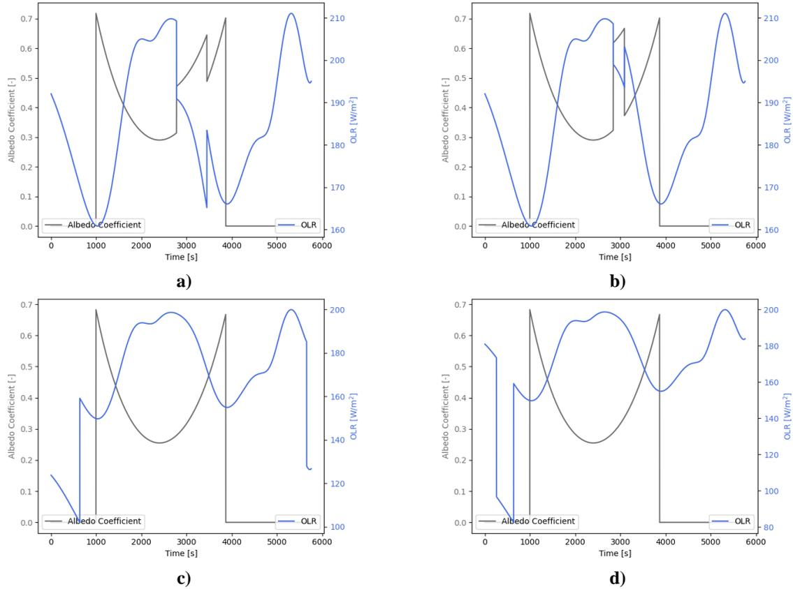
**Figure 8. Albedo and OLR profiles for the a) coldest and b) hottest worst-cases of the  $t_c = 300$  s and c) coldest and d) hottest worst-cases of the  $t_c = 1100$  s.**
