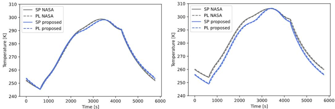
**Figure 11. Case 2 (coupled nodes) thermal model temperature response for the coldest (left) and hottest (right) worst-cases using NASA and time-dependent proposed criteria.**
