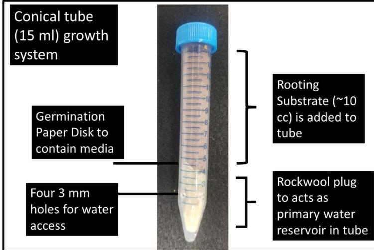
**Figure 2** Components of the conical plant growth tube used in the whole plant lettuce bioassay.
