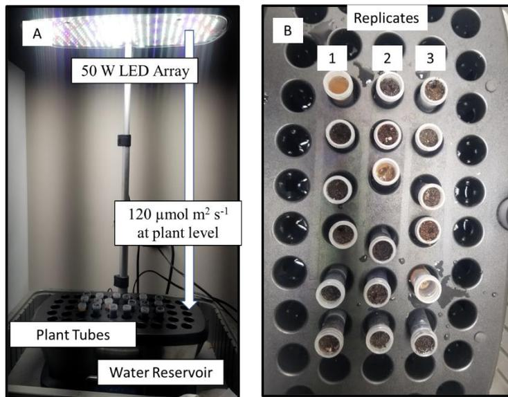
**Figure 3** A: Test stand as configured with three replicates of conical growth tubes, 50-Watt broad spectrum LED lighting and common 5 Liter water reservoir of the AeroGarden™ test stand. B. Conical tubes with media were randomized in the
