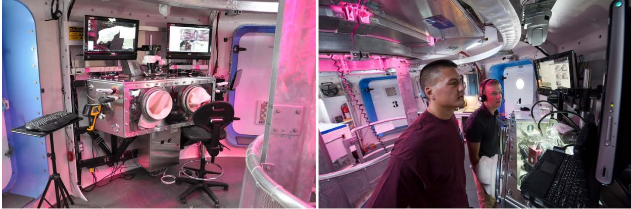
Figure 6. (Left) The GeoLab bay layout from the Desert RATS analog mission in 2011 showing the sample glovebox, multiple touchscreen displays, a microscope (above), other cameras and instruments, and control box below. (Right) Crew members at the workstation, including strained body posture for the glovebox operator. The addition of a seat (left) likely helps with glovebox ergonomics, but may increase the look angles to the monitors. 24
