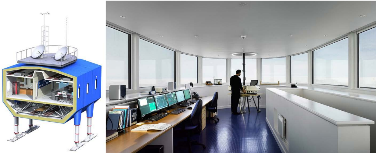
Figure 8. (Left) Cross-sectional cutaway view of a Halley VI standardized module showing internal structure, the habitable area, and the stilts and skis used for relocation. (Right) The meteorological observation deck offers panoramic views and daylight. 31
