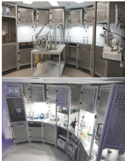
Figure 7. MaMBA science lab mockup with modular racks to support different science configurations. 27
