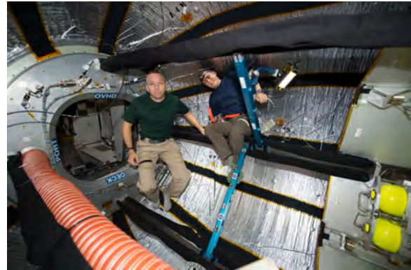
Figure 2. Interior of BEAM inflatable module on ISS
