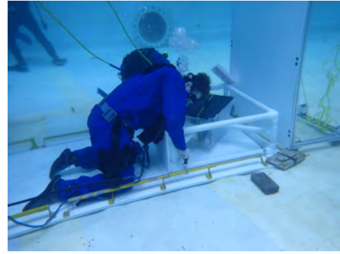
Figure 16. Images from the lunar test. Divers are securing down the equipment, representing the second step in the testing procedure.
