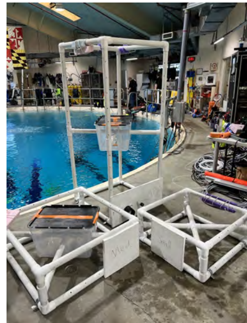
Figure 10. Test equipment used for microgravity and lunar tests. The small, medium, and large PVC structures are displayed.
