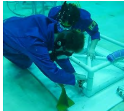
Figure 14. Divers securing the small payload simulator during the microgravity test, representing the second step in the testing procedure.
