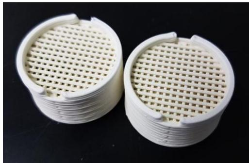
**Figure 3: Printed MultiSORB 13X zeolite adsorbent lattices (1" diameter and ½" height)**
