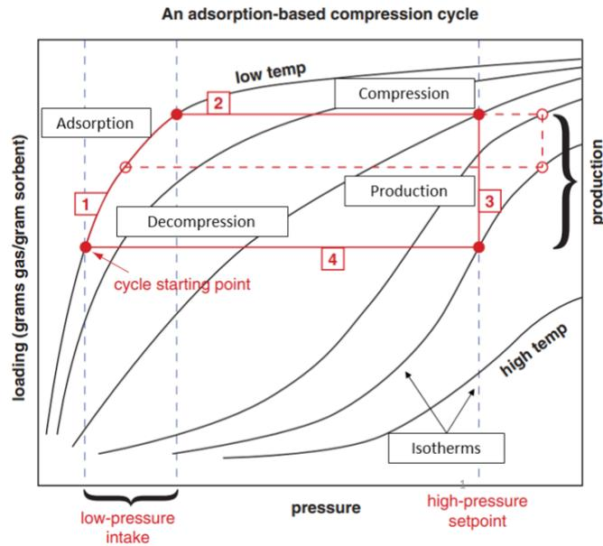
**Figure 2. Operating cycle for an Air-Cooled Temperature Swing Adsorption Compressor<sup>6</sup>**
