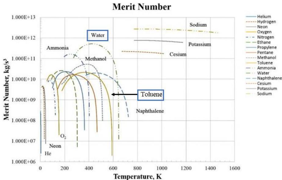
**Figure 7. Merit number of different working fluids<sup>30</sup>**
