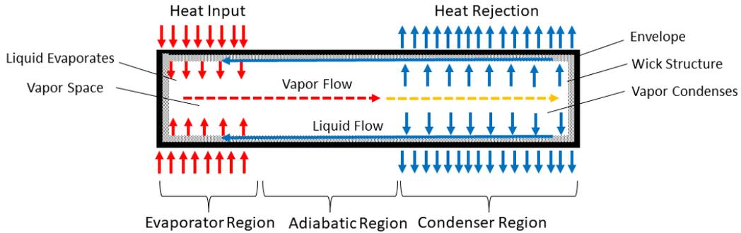
**Figure 5. Heat pipe and vapor chamber working principles diagram**
