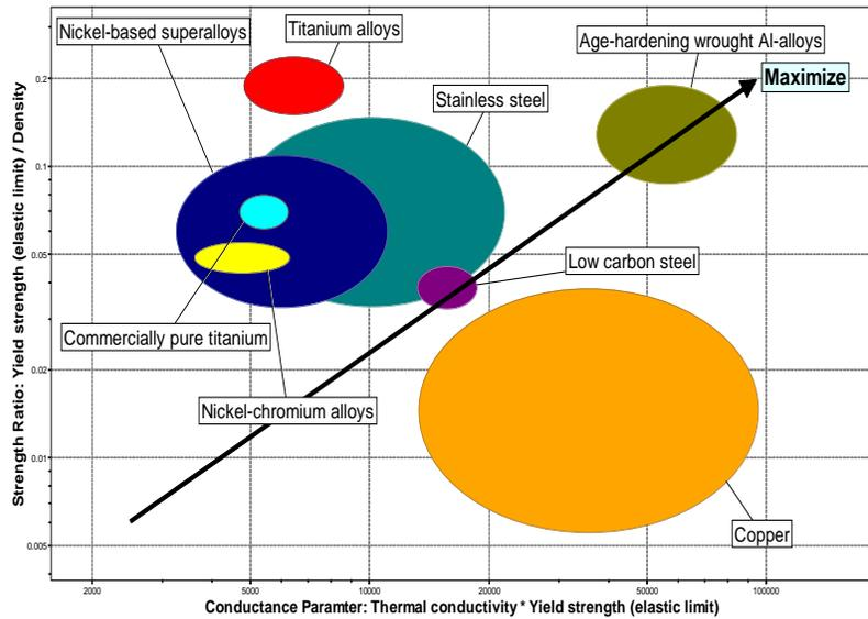
**Figure 8. Ashby chart for strength ratio and conductance parameter**
