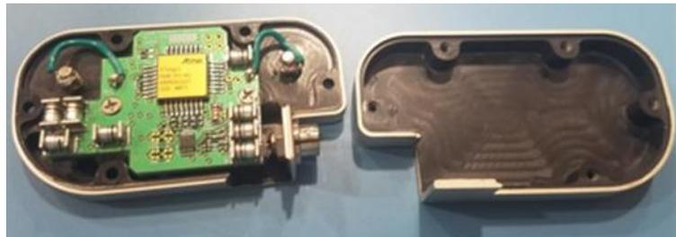
**Figure 4. WHRM Electronics Module, internal**
