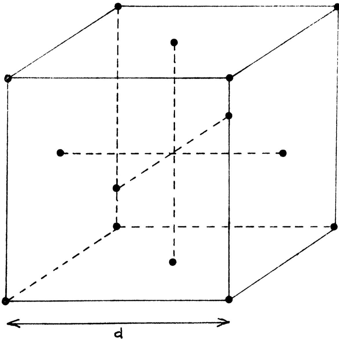
Fig. 1 Face-centered Cubic Compound Cell
