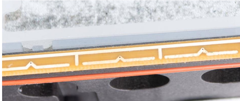
Figure 8. Image of BPA leak sensor after several rounds of cleaning activities showing significant reduction in corrosion. Photo credit: NASA ISS Imagery Online.
