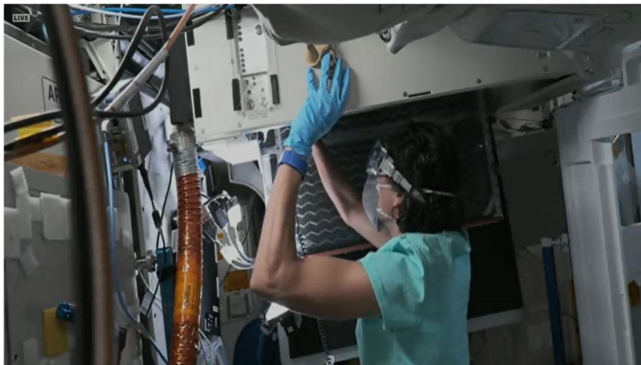
Figure 7. Image of BPA leak sensor cleaning activities showing ISS crewmember Jasmin Moghbeli working on the BPA. Photo credit: NASA ISS Imagery Online.
