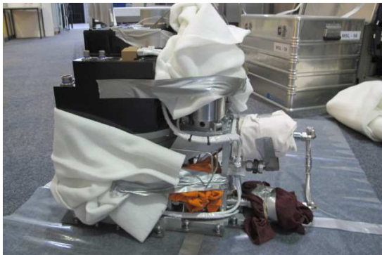
Figure 6: T-shirts placement (in contact with delicate parts of WPA)
