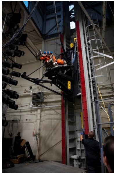
Figure 2. The VDT at WPAFB. The photo shows a human subject being raised to the required drop height 5 .
