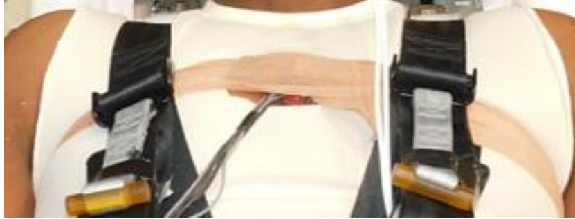
Figure 4. The chest accelerometer was affixed to subjects with double-sided carpet tape through a hole in their shirt. The accelerometer was wrapped in athletic tape around the torso to provide more stability.
