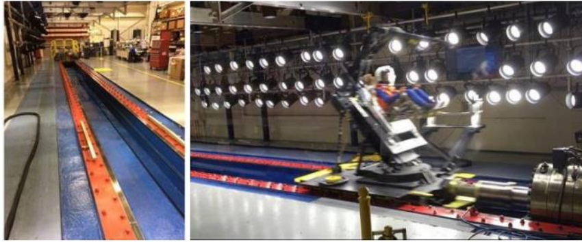
Figure 1. The HIA at WPAFB. The photo on the left shows the sled track, and the photo on the right shows an ATD suited test 4 .
