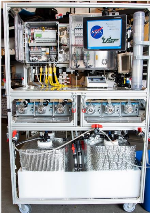
Figure 1. Organic Processor Assembly unit. The biological portion (buffer tank, reactor 1, reactor 2) sits in the bottom of OPA. The tubular membrane sits in the upper right-hand corner where it is easily assessable.
