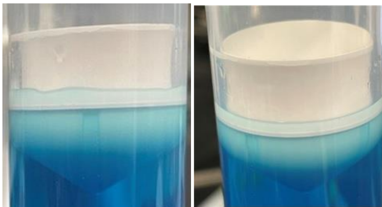
Figure 11a (left). Leakage in the piston channel after its insertion, tank not pressurized.
