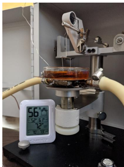
Figure 5. Temperature-controlled IL surface tension measurement setup.
