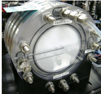
4 stack membrane-type water/gas separator.
