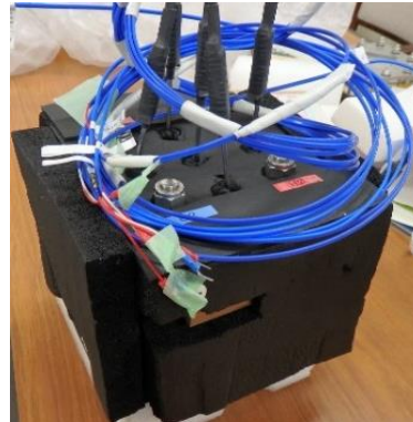
10 cells water electrolyzer
