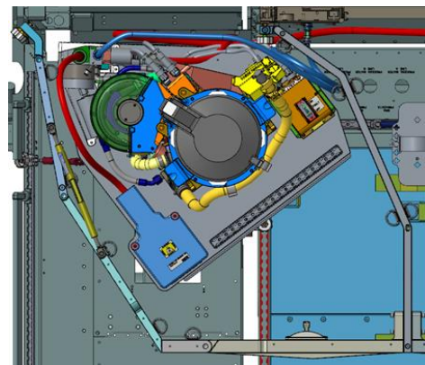
Figure 7. Toilet Mounting Adapter inside Toilet Stall with Hardware Mounted (Note: Mounting Adapter is shown in grey).
