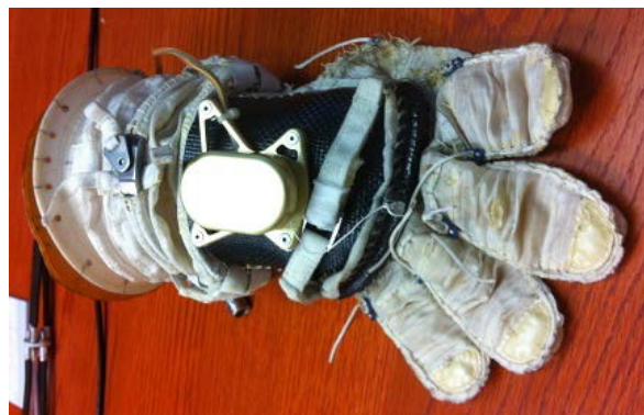
Figure 1. Existing exoskeleton EVA glove with electromechanical actuation.
