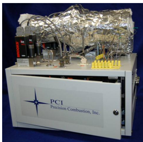
Figure 8. Photo of the integrated SDU prototype system with the downselected Sabatier reactor and all necessary BOP components.
