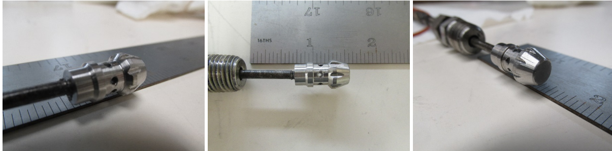
Figure 4: Images showing stainless steel nozzle-mixing chamber with six radial holes located just above the circumferential collar, which serve as the ejection ports for fuel entering from the steel fuel supply tube attached at the base.
