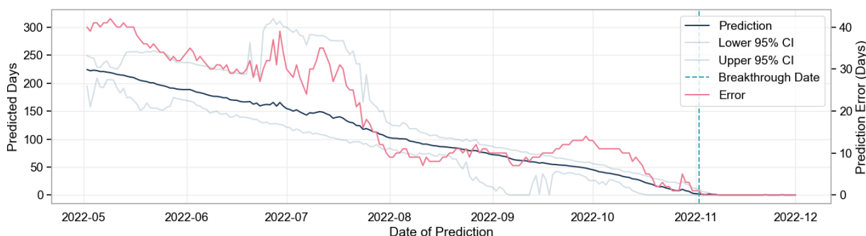
Figure 3. Plot showing the WPA MFB RUL prediction (in number of days remaining until first ionic breakthrough) at each day in 2022.
