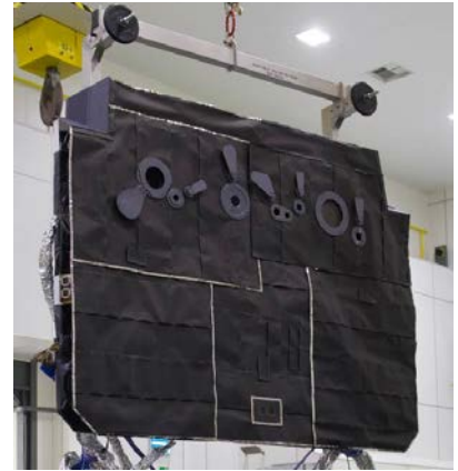
Figure 1. FDMs installed in SOLO Heat Shield (ESA )
