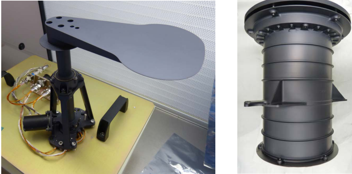
Figure 12. Door mechanism and Feedthrough of FDMs (Sener copyright)
