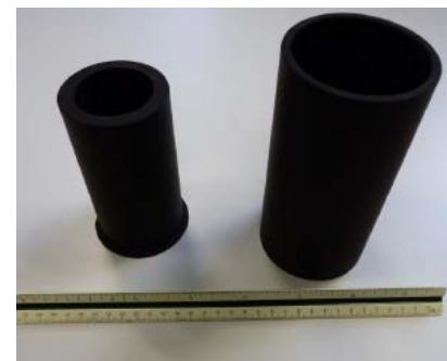
Figure 5. Coating application verification with dummy models representing the Feedthroughs geometry (Sener copyright)
