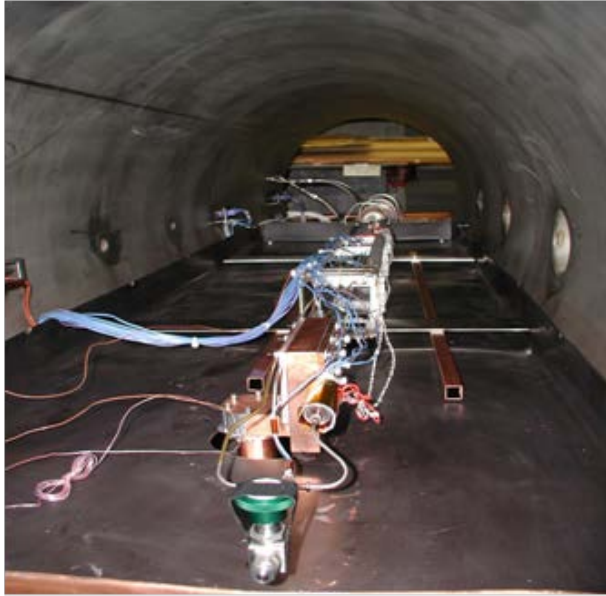
Figure 9. Hydrogen CLHP in Thermal Vacuum Chamber
