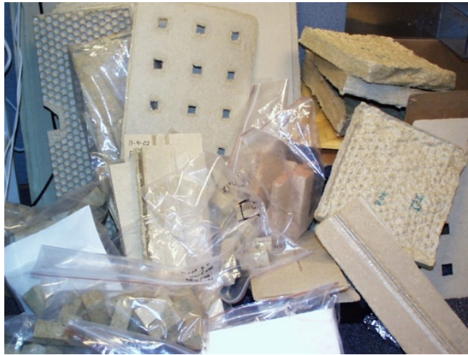
Figure 3. “Surplused” structures (root/shoot barriers, seed plugs, panels, truss members, and fiber mats) derived from formed wheat fiber. These materials were reprocessed into new structures.
