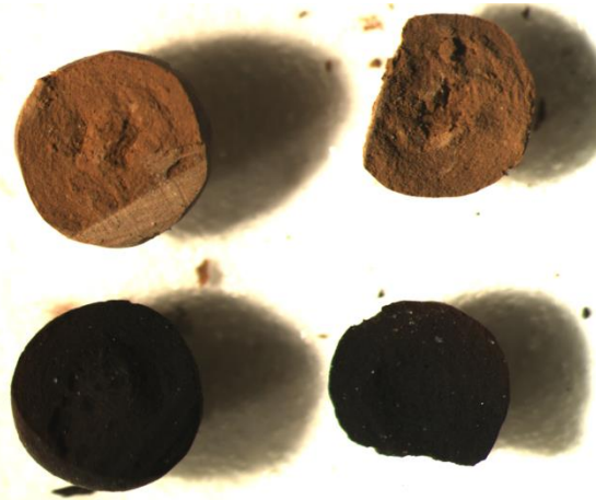
Figure 7: Micrograph of bisected discolored 13X sorbent beads.
