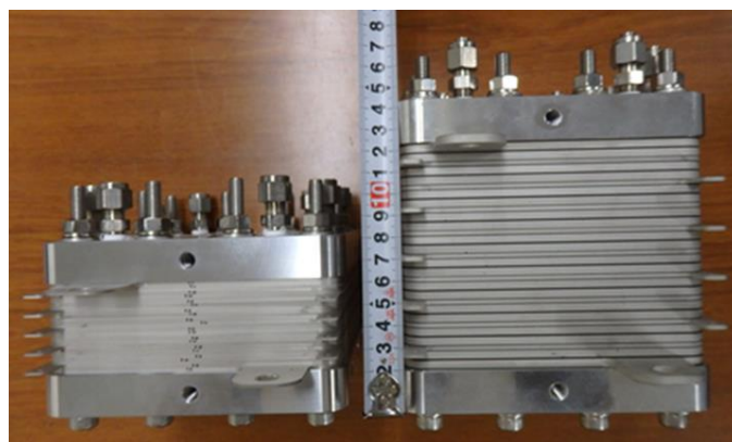
Figure 3. Water electrolyzers of the full-scale model (left) and the sub-scale model (right).
