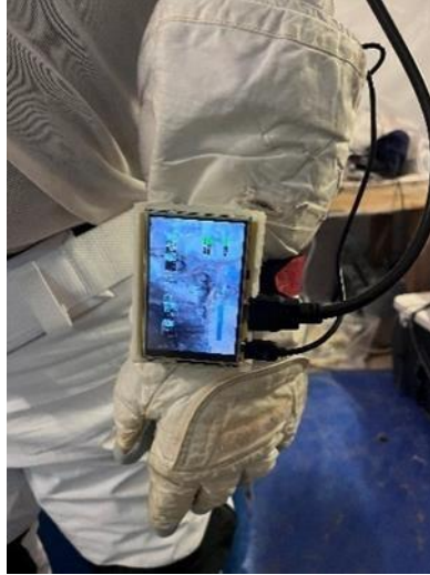
Figure 2: Tethered display mounted on an EVA glove
