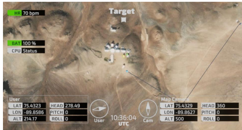
Figure 5: Birds eye view rendering of the HMPRS Base camp along with navigation, consumables and biometric data displayed
