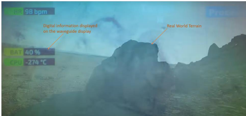
Figure 4: Rendering of in field view through waveguide displays
