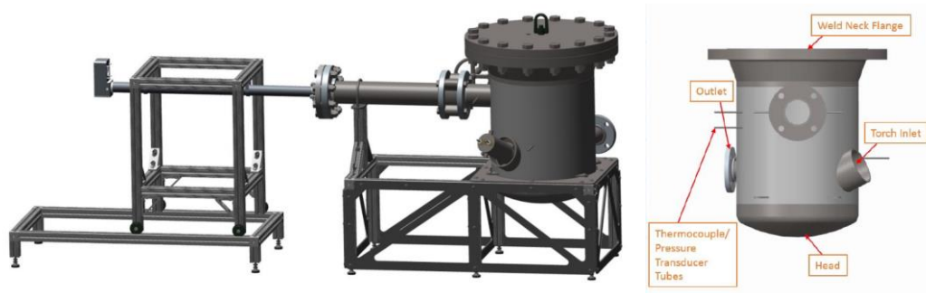
Figure 2. MPG model of feed system, reactor body, and reactor body with labels.
