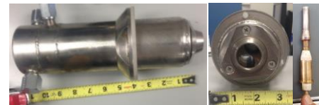
Figure 4. Plasma arc torch housing. Left: Torch side view, Middle: Torch plume exit view, Right: Electrode.
