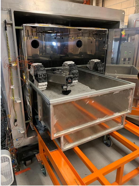
3 4. One of the two regolith boxes with a lunar rover prototype being loaded in the Dusty Thermal Vacuum Chamber at MTU-PSTD. Credit: Paul van Susante.
