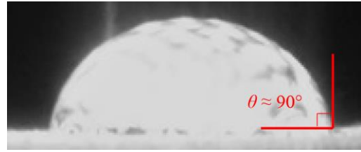
Figure 3. Contact angle between water and sintered copper particles.
