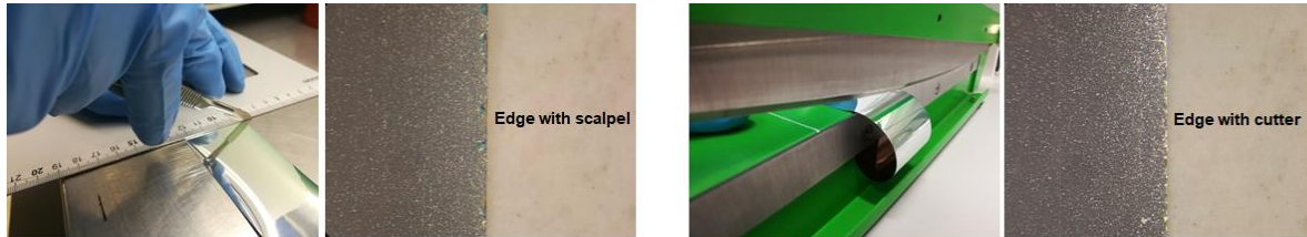
Figure 9. Cutting operations and coating edges under the microscope 40×.
