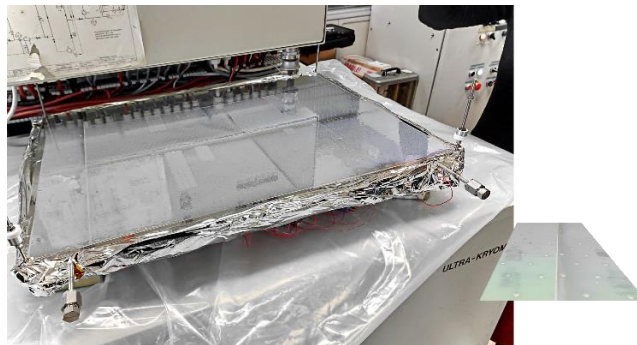
Figure 10. Application test results. Left: Biosmart radiator covered with FF-OSRs. Right: surface detail.
