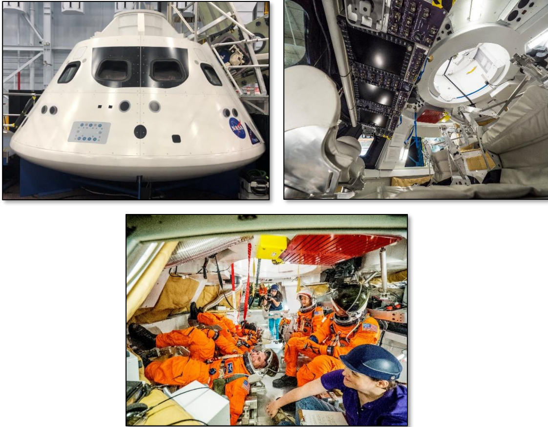
Figure 5. Examples of a hi-fi mockup from the Orion capsule at the NASA JSC Space Vehicle Mockup Facility (SVMF), depicting its use during a crew survivability HITL test.
