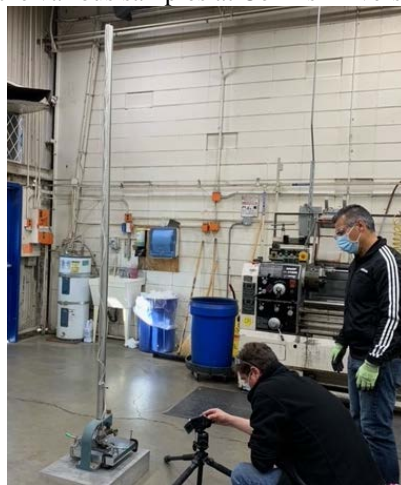
Figure 9. Drop Test Stand. Patrick Nolan and Roberto Ramos film the test using a high speed camera.
