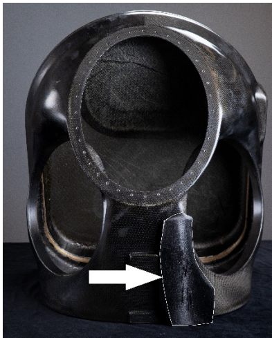
Figure 4. Armor Prototype attached to the HUT demonstrator. This AM armor (outline was created to demonstrate how the armor piece would fit onto the HUT).
