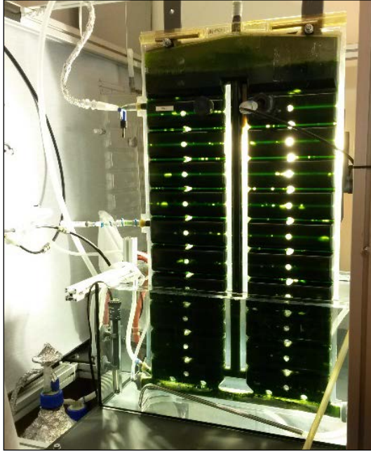
Figure 5. Subitec® Reactors at IRS-lab, used for the scale-up process
