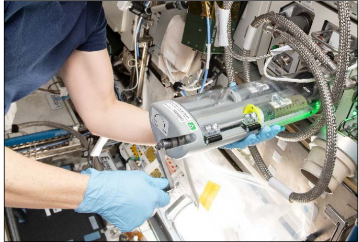
Figure 10. Start Medium insertion using the Liquid Exchange Device at GMT157. Credits NASA
