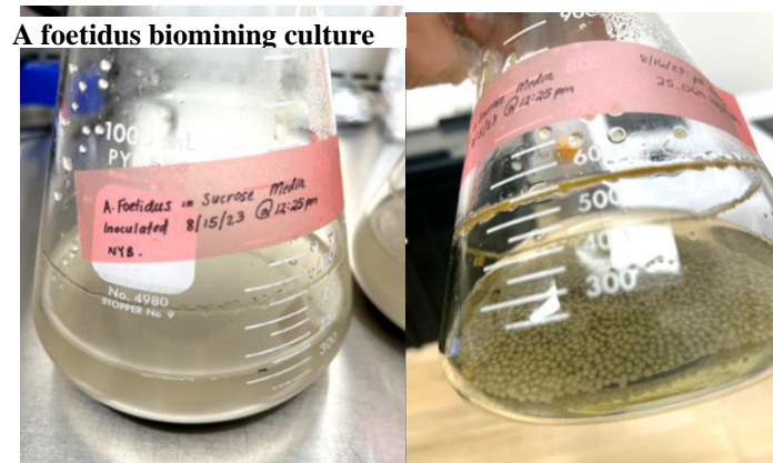
Figure 2a and 4b. Pictured on the left 4a A. foetidus fungal culture after addition of lunar simulant (day 1). Pictured on the right 4b A. foetidus fungal culture with lunar simulant three days after addition of lunar simulant.
