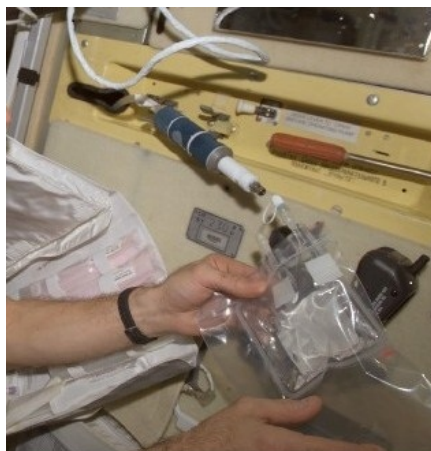
Figure 3 - SVO-ZV stored water dispenser. Collection of water sample from SVO-ZV (NASA/JSC Photo #ISS006E08617)
