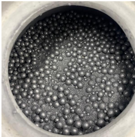
Figure 3. Ball-Milled Aluminum Inside Jar with YSZ Balls
