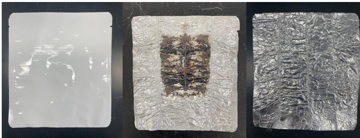
Figure 2. Original food packaging material (left), uncleaned aluminum layer post-TtG process (middle), and Alconox®-cleaned aluminum sheet (right)
