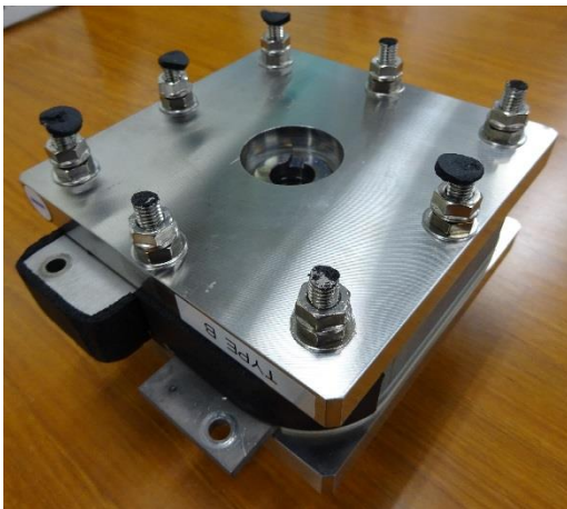
Figure 4 JAXA's improved single water electrolysis cell.
