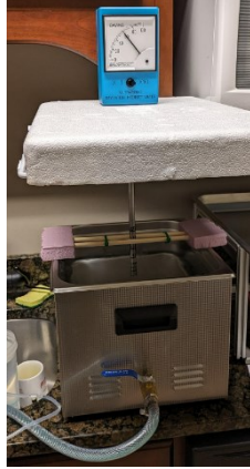
Figure 6. Measuring the ultrasonic cleaner cavitation intensity for different bath depths.
