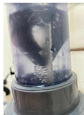
Figure 2. Hydrogen gas bubbles on a titanium plate.
