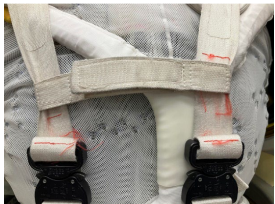
Figure 2: Interior view of the HUT from the top showcasing shoulder strap attachment points (top), shoulder strap sizing (bottom).
