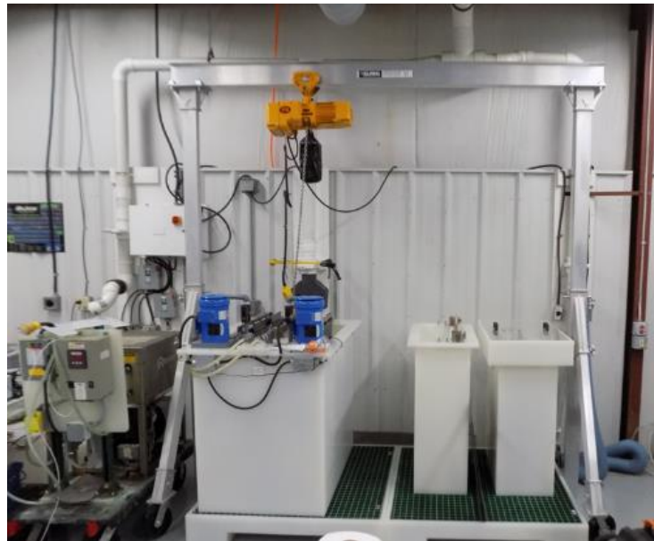
Figure 10. The scale-up deposition system for graphene-Cu hybrid foil fabrication.
