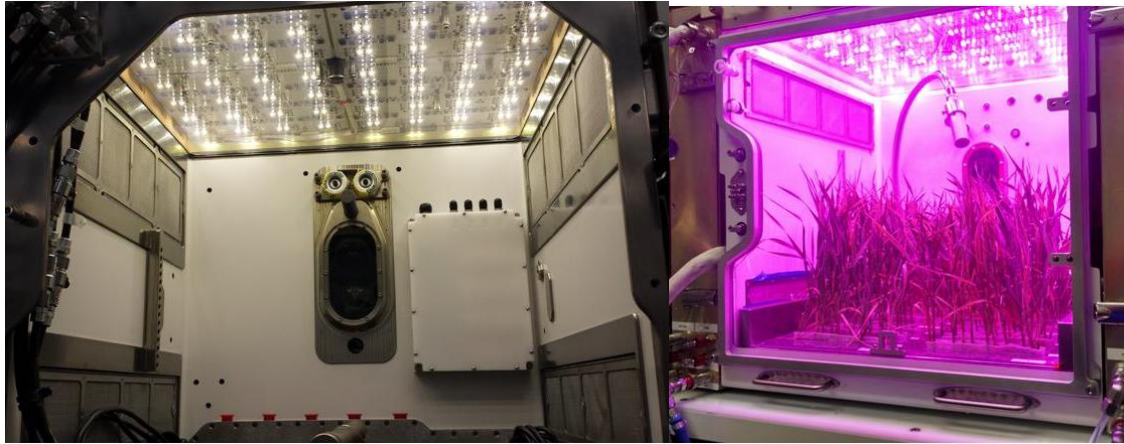
Figure 6. L>R. GLA with the broad spectrum (white) LEDs powered on; top view camera is visible at the intersection of the four light panels. GLA with red and blue LEDs powered on during plant growth test. Infrared thermometer for measuring leaf surface temperatures is shown on a flex arm at top of plant canopy.
