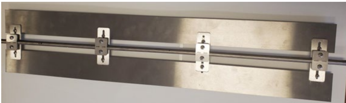
Figure 4. Combined Attritor Arm Catalyst Delivery Assembly
