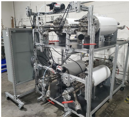
Figure 6. Pressurized 4-CM CFR System on its Test Stand in a 2x2 Array Delivered to GRC in February 2024
