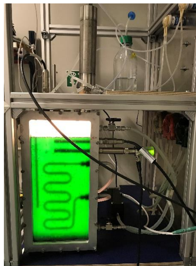
Figure 7. Improved configuration of the PBR. To avoid condensate on the gas sensors and the PTFE filter membrane, a gas drying unit is attached to the gas outlet of the PBR. In addition, the DOX and OD sensors are mounted on the side to avoid measurement interferences due to gas bubbles. Shown here is the PBR after 160 hours with an OD_{750} of 1.37.
