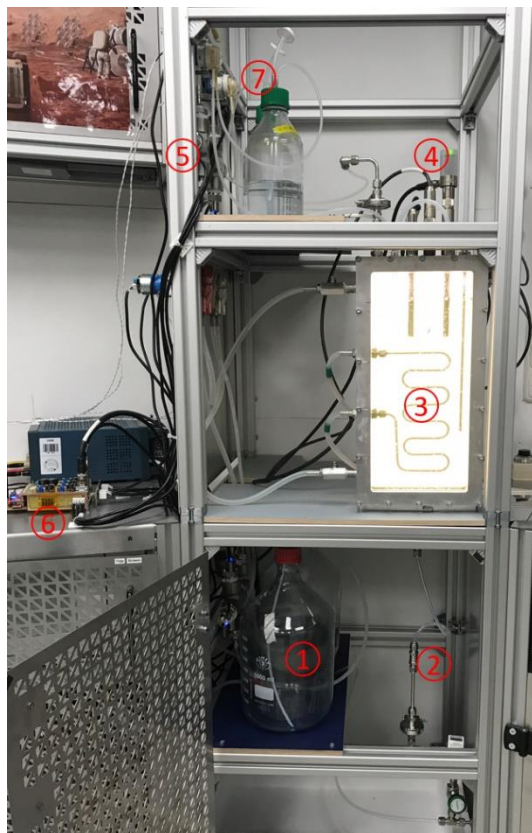
Figure 2. Experimental set-up including the first configuration of the PBR and its periphery. With the help of the peristaltic pumps, either fresh medium is pumped into the reactor or cell suspension is pumped out of it, into the harvest bottle (1). The air for gas exchange and mixing is fed into the PBR from the bottom (2). Cooling/heating water is pumped through the bent stainless steel pipe (3) for temperature regulation. During the process, the parameters in the cyanobacteria suspension (4) and in the gas outlet (5) are measured continuously. All sensors and actuators are connected to the data processing unit (6). Either an acidic solution or a basic one (7) can be pumped into the PBR for pH regulation.
