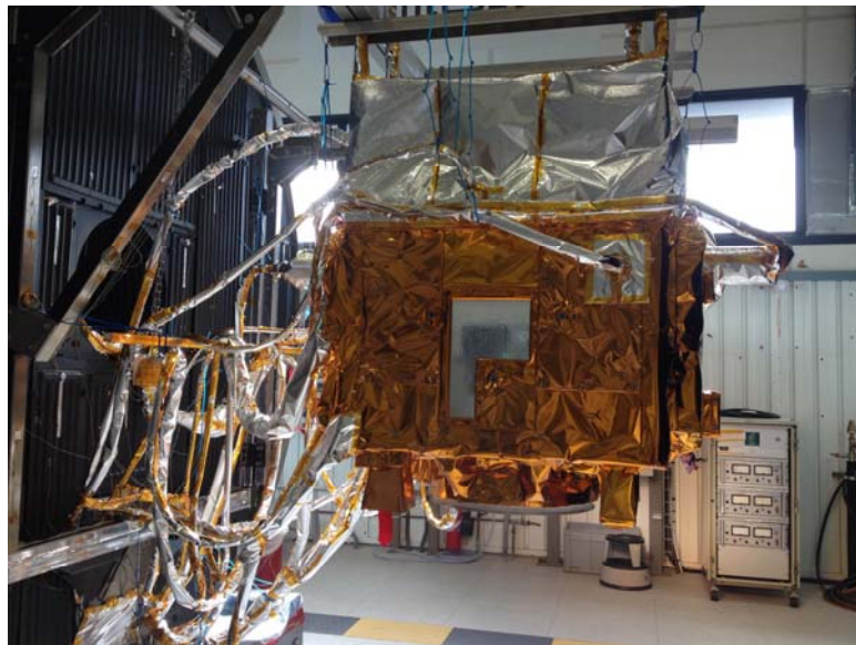
Figure 3. MICROSCOPE thermal vacuum testing configuration.
