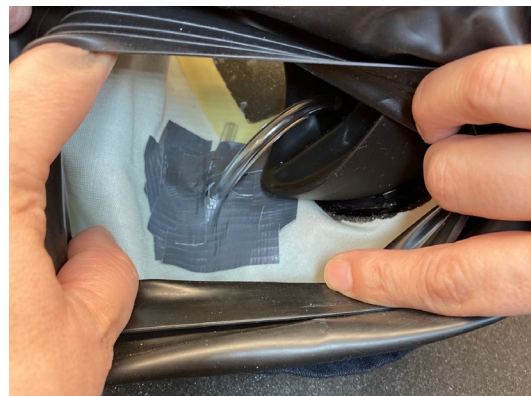
Figure 2. Sampling tube breaching the nosecup and adhered to the inside of the hood.
