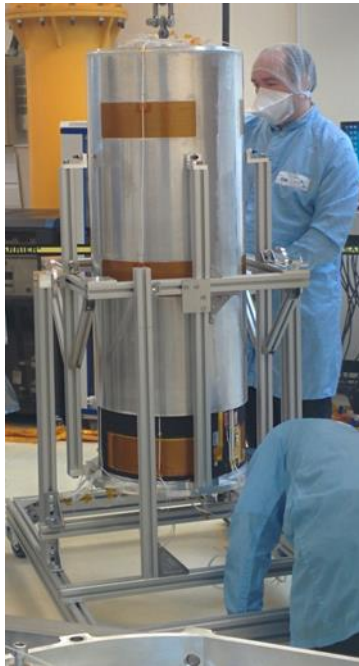
Figure 2 Assembly of BBM at RAL Space. Heaters are clearly displayed on both the black coated inner cavity and the aluminum radiation shield.
